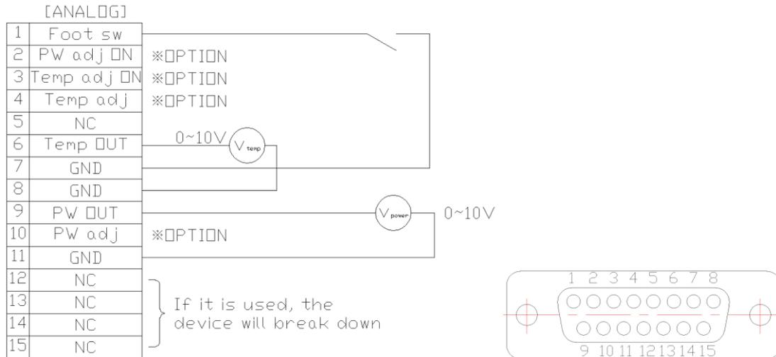
● It is necessary to use a Shielded Cable and a ferrite core for this connection.
