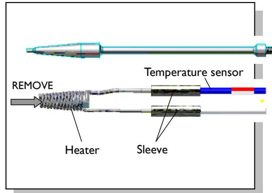
6. Check the contact between the tip and the heater. If the heater position is too much forward or if the heater is pressing too much on the tip, adjust so they are not in contact with each other. The guideline for adjustment is to have the end of the heater coiling and the beginning of the straight section of the tip matching.
