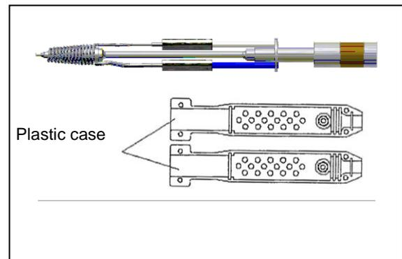
4. Pull the sleeve until the heater connection points became visible, and remove the heater with caution not to bend it.
